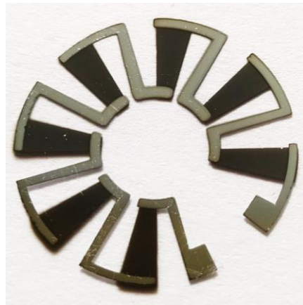
Fig. 9. Sputtered CoSi side of the device in the form of a camomile
